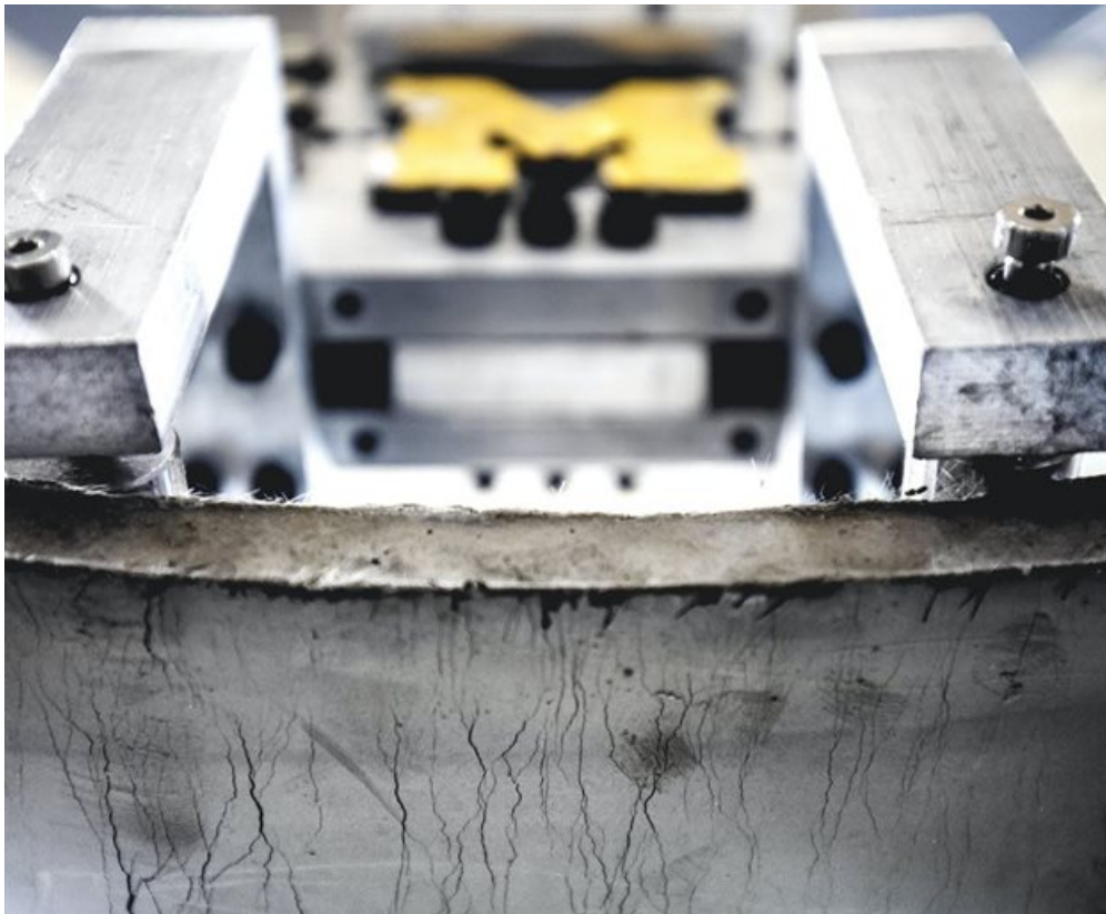
Bendable concrete created at the University of Michigan allows for thinner structures with less need for steel reinforcement. Joseph Xu/University of Michigan College of Engineering
