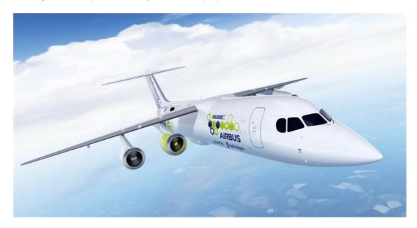
The E-Fan X hybrid-electric technology demonstrator is anticipated to fly in 2020 following a comprehensive ground test campaign, provisionally on a BAe 146 flying testbed, with one of the aircraft's four gas turbine engines replaced by a two-megawatt electric motor. Provisions will be made to replace a second gas turbine with an electric motor once system maturity has been proven.
