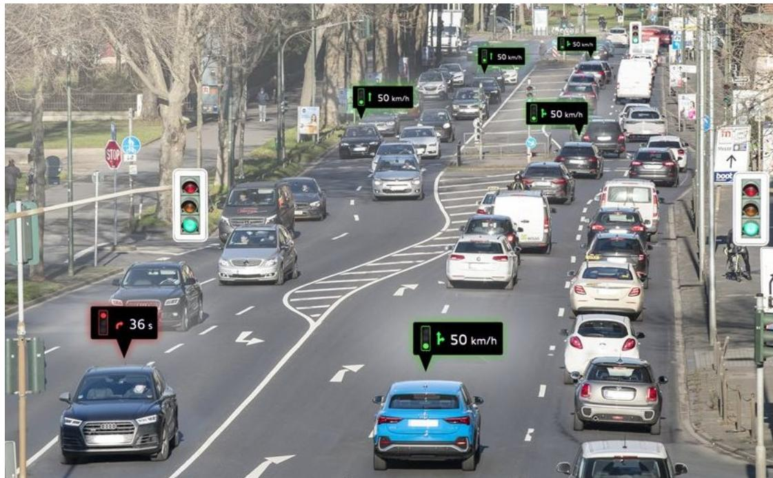
Audi Traffic Light Information is a vehicle-to-infrastructure service that increases efficiency, convenience and safety on roads. Most of the intersections in Düsseldorf, approximately 450 out of a total of some 600 installations, will be networked.
