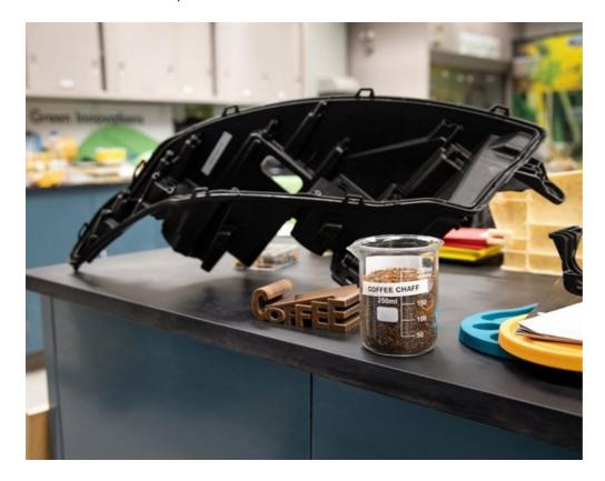
The chaff composite meets the quality specifications for parts like headlamp housings and other interior and under hood components. The resulting components will be about 20% lighter and require up to 25% less energy during the molding process. Heat properties of the chaff component are significantly better than the currently used material, according to Ford. This is the first time Ford has used coffee bean skins to convert into select vehicle parts.
